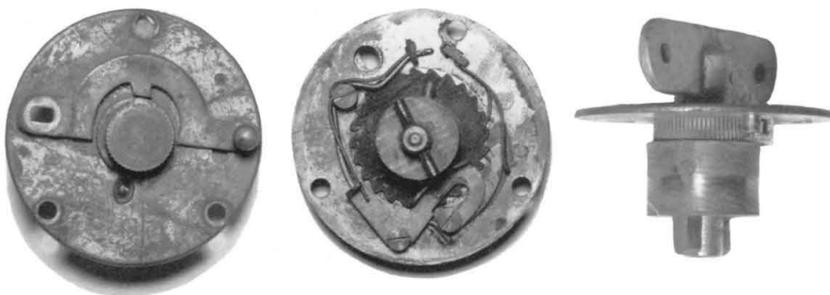
Above: Film winding and counting mechanism from roll-holder.
