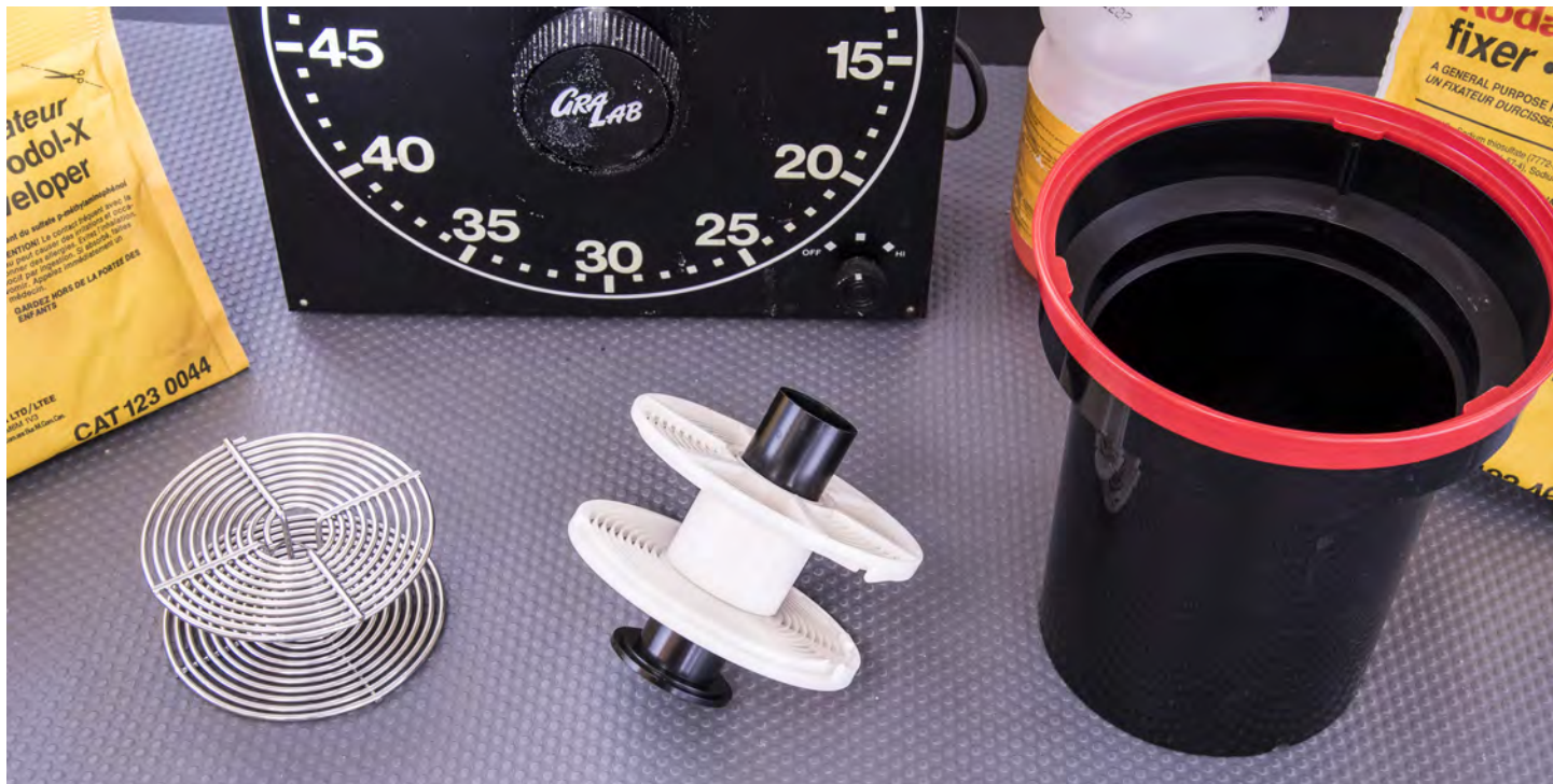
Front: a stainless spiral for a stainless tank (below), the plastic Paterson reel and a snazzy red-rim Paterson tank.
