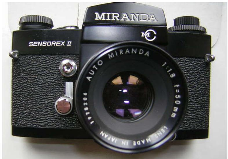
Miranda did not make their own lenses and had to rely on other manufacturers to supply them. All their SLR cameras, except the dx-3, had interchangeable pentaprisms, and a unique dual lens mount; an external bayonet mount or a 44mm thread mount within the mirror box.
